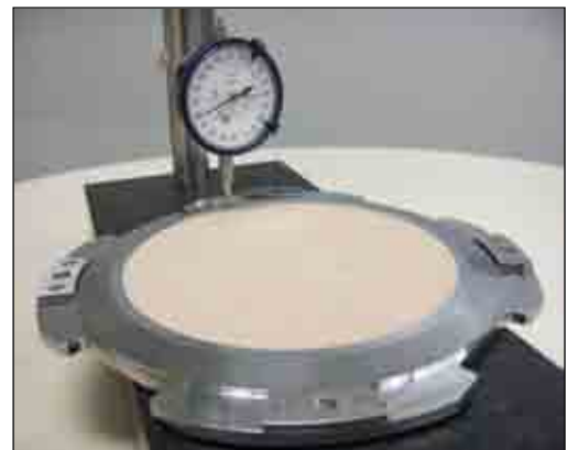
Inspection of wafer chuck's parallelism 18-211-050
