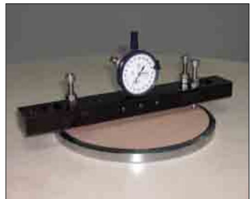
Inspection of wafer chuck's flatness 18-211-010
